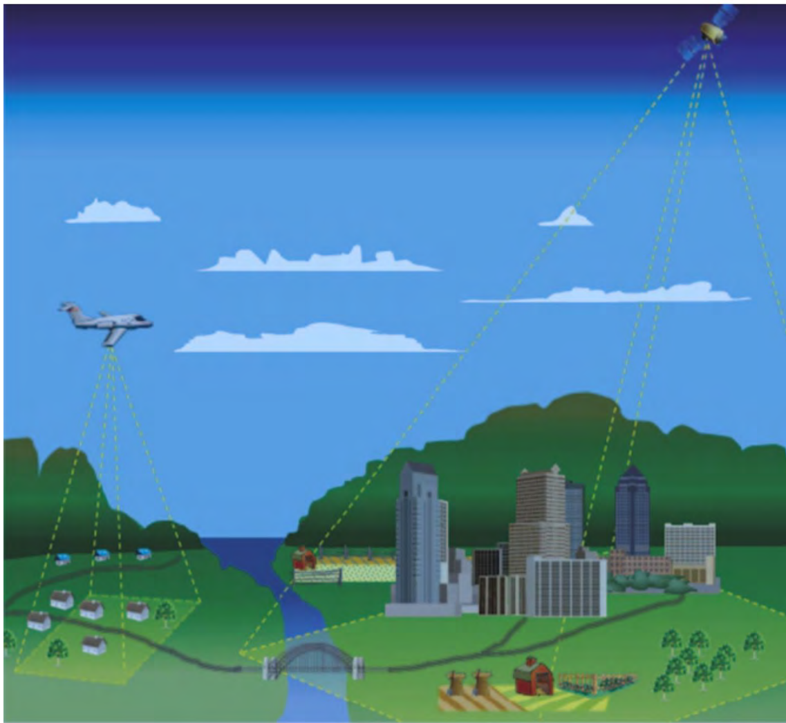
Fig: An illustration of the remote sensing concept: An instrument (i.e., sensor or scanner) mounted on an aircraft or satellite records information about objects and/or areas on the ground. Typically, these data are spectral in nature, meaning that they document the amount of electro- magnetic energy associated with the targeted objects and/or areas. The extent, or footprint, of the geographic area captured in a single-sensor scene depends on the sensor's design and the altitude of the aircraft or spacecraft on which it is mounted.
